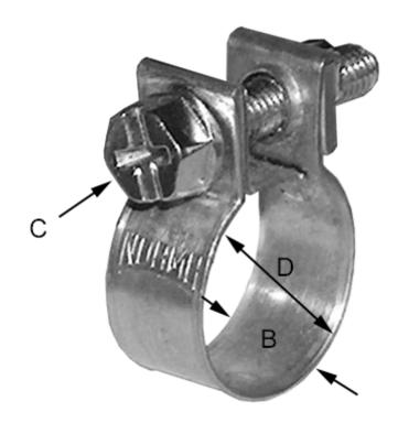
C (screw type) = C7 hexagon screw sw 7, cross-headed Diameter D = 9,5-15,5Width B = 9
